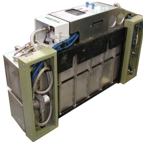
Coal loco metal-hydride storage (complete)
